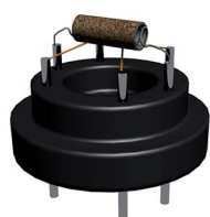
Fig. 1 Schematic structure of the completed gas sensor.
