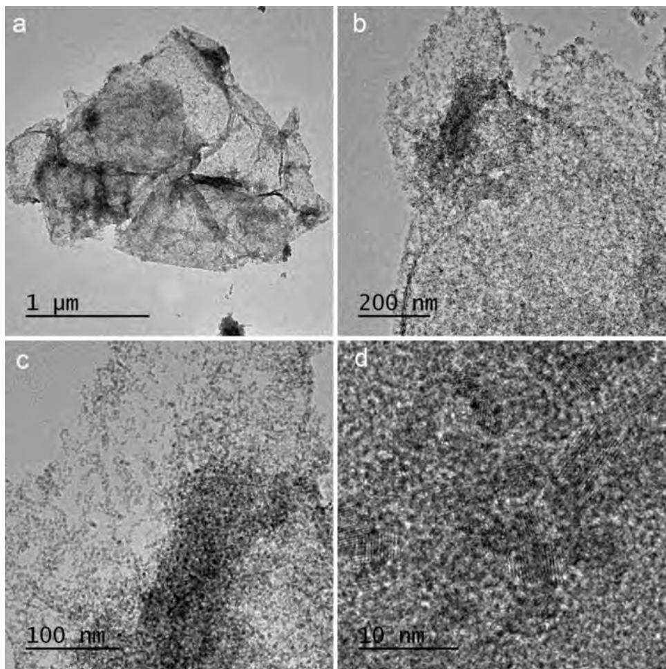
**Fig. 6.** The TEM images of  $\text{SnO}_2/\text{S-rGO}$  hybrids.
