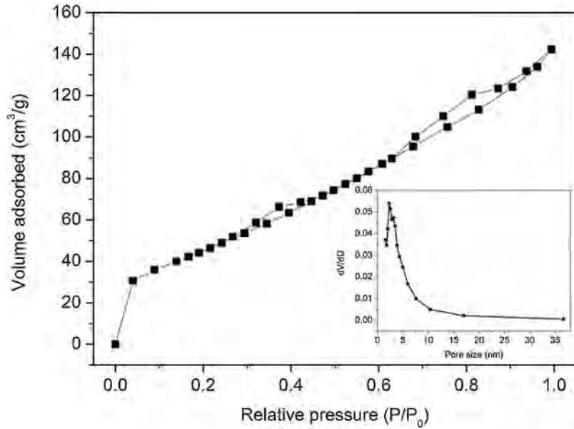
**Fig. 7.**  $\text{N}_2$  sorption isotherms of  $\text{SnO}_2/\text{S-rGO}$  hybrids. Inset shows the corresponding pore size distribution curve.
