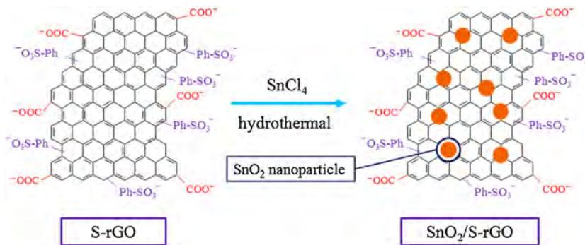
**Fig. 1.** A scheme to illustrate the modification of S-rGO with  $\text{SnO}_2$  nanoparticles by hydrothermal synthesis method.
