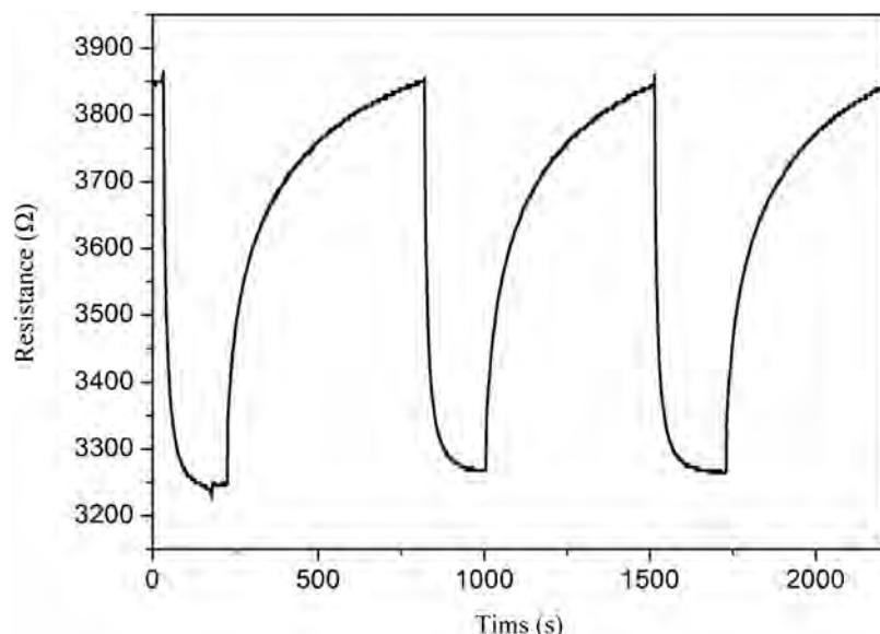
**Fig. 10.** The reproducibility of temporal response of  $\text{SnO}_2/\text{S-rGO}$  hybrids exposed to 5 ppm  $\text{NO}_2$  at room temperature.
