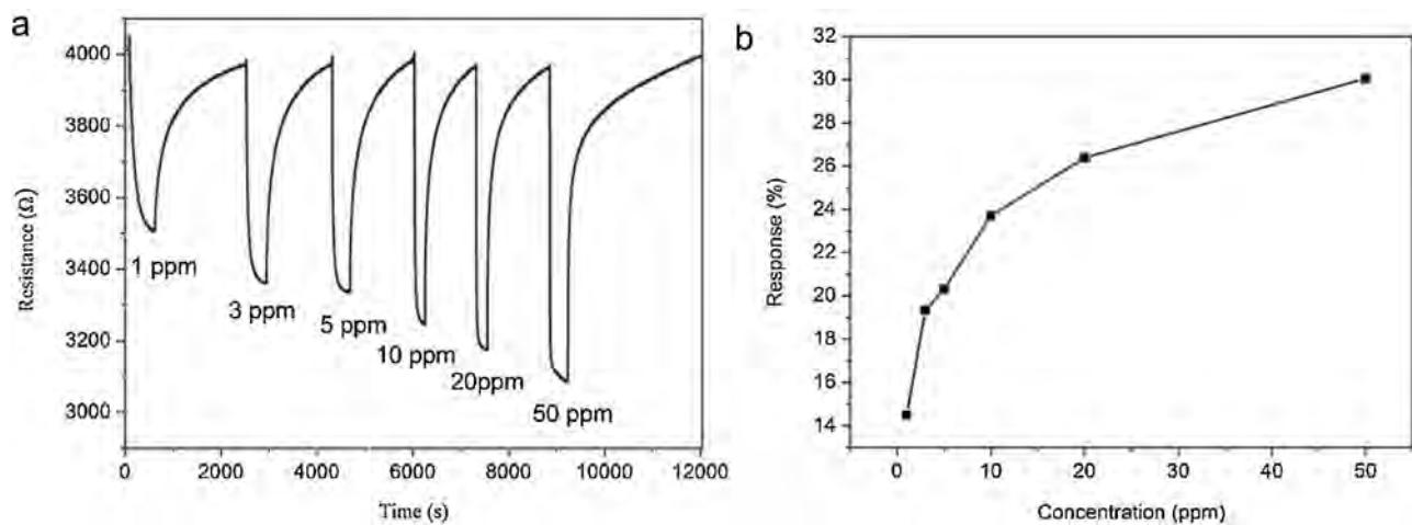
**Fig. 8.** (a) Dynamic sensing responses of  $\text{SnO}_2/\text{S-rGO}$  sensors upon exposure to  $\text{NO}_2$  gas with concentrations varying from 1 to 50 ppm, and (b) the corresponding response variations of  $\text{SnO}_2/\text{S-rGO}$  sensors as a function of  $\text{NO}_2$  concentrations.
