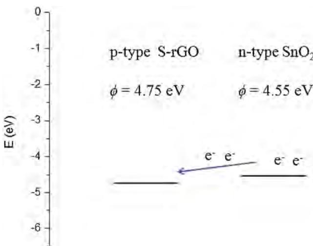
Fig. 12. The scheme to illustrate the electrons transfer progress between S-rGO and  $\text{SnO}_2$  during the  $\text{NO}_2$  sensing.
