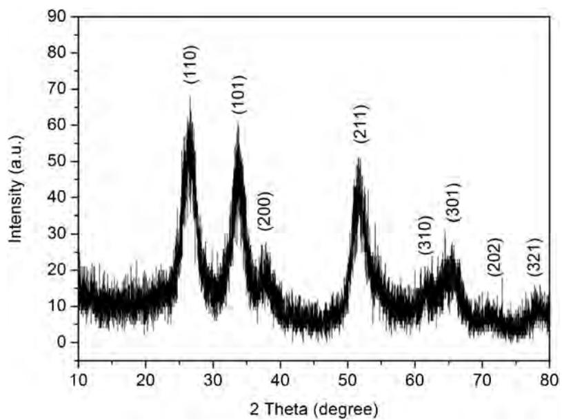
**Fig. 4.** XRD pattern of SnO<sub>2</sub>/S-rGO hybrids.
