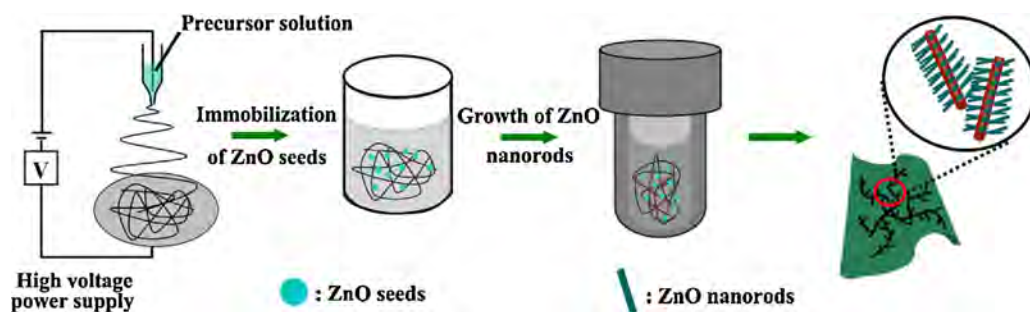
Fig. 1. Strategy for growing ZnO nanorods onto \text{TiO}_2 nanofibers surface using hydrothermal method.
